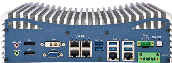
*Visual Inspection Image - the rear picture of the Eagle Eyes-AIH for the visual inspection (shows PoE ports):
